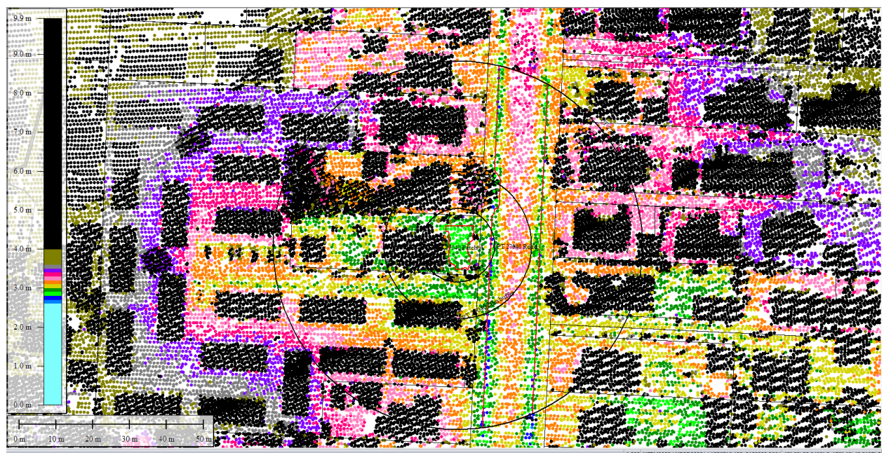
Figure 48: Ground surface elevation averaged over 50-m buffer for Road for Sep 5, 2010 LiDAR survey.
